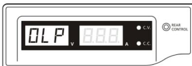
To reset this warning, switch off the unit and remove all loading.
